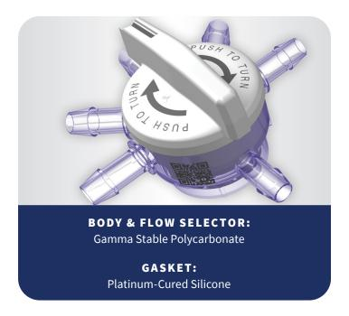
The barbs are sized to support 3/8" (9.5 mm) ID tubing and are designed specifically to work with industry preferred silicone and TPE style tubing. The manifold is made from industry standard polycarbonate with a platinum-cured silicone internal seal. The only material that will come into contact with the drug product are the polycarbonate housing and the silicone seal.
